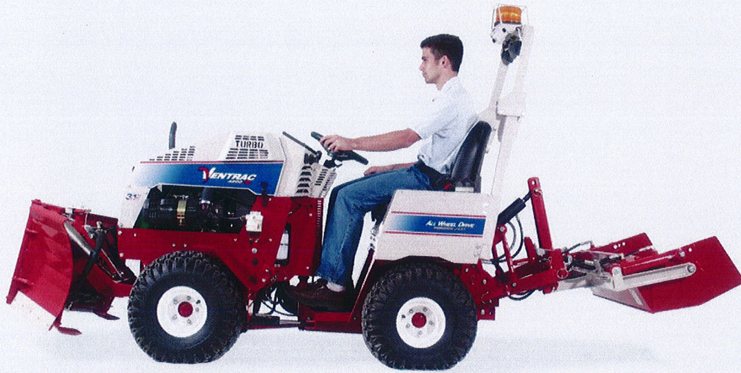
Rear mounted attachment on 3-N-1 Adapter shown with optional Hydraulic Top Link
